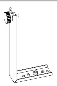
This accessory provides 2 welded M5 nuts and 1 welded M10 nut. (It should always be used along with the FS0081-001.) This adapter allows the cabinet to be fixed on the wall, ceiling or on a stand using the FS0081-003
